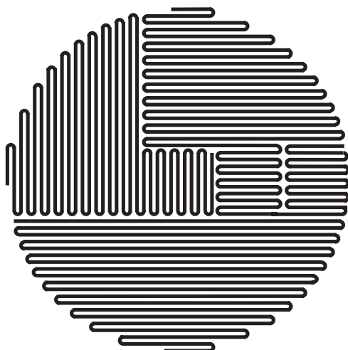
Figure 7. Top view of a hypothetical nanomesa showing several chain-folding structures that may be present. Some of the chains may extend beyond the perimeter and return elsewhere, leaving amorphous loops similar to those found on the faces of lamellar crystals [11, 12].
